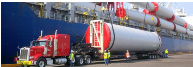
Discharging tower sections at the Port of Brownsville
